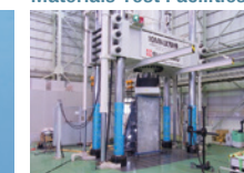
CFRP panel compression test
