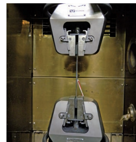
積層複合材の引張強度試験 Tensile Strength Test of Laminated Composite
