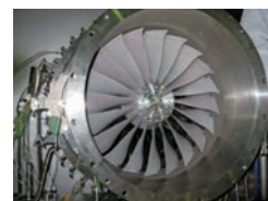
高効率ファン空力性能試験 High Efficiency Fan Aerodynamic Performance Test
