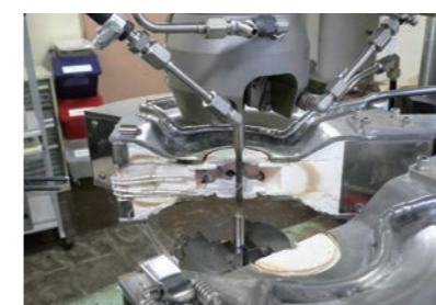
先進超合金の高低温低サイクル疲労試験 High Temperature Low Cycle Fatigue Test of Advanced Superalloy
