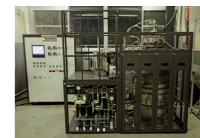
先進複合材の高温酸化加速試験 Accelerated Oxidation Test of Advanced Composite Material
