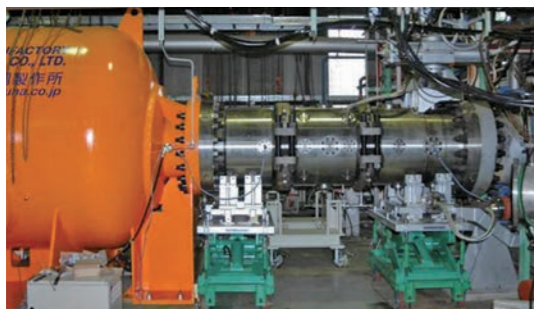
高温高圧燃焼試験設備 High Temperature & Pressure Combustion Test Facility. Inlet Temperature & Pressure (Max): 1000K, 5.0MPa, Air Flow Rate(Max): 4.0kg/s, Fuel: Kerosene, Methane gas.
