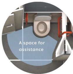
A space for assistance on the side of the toilet seat
