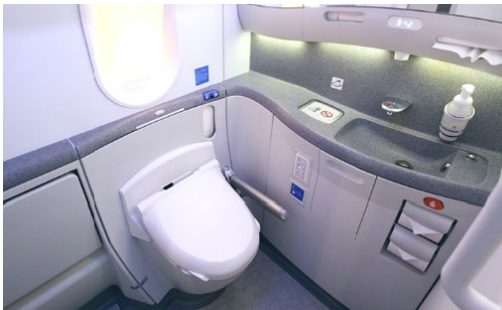
Conventional aircraft lavatories have no space for two caregivers to assist PRMs.
