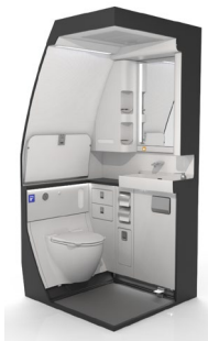
Conventional aircraft lavatories have no space for two caregivers to assist PRMs.
