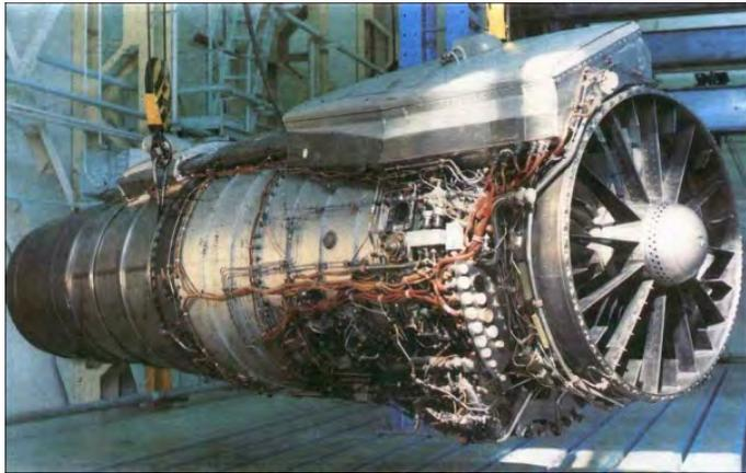
Cryogenic gas fuel Tupolev-155 test bed. Flight demonstration of cryogenic methane and hydrogen for one of its three engines
