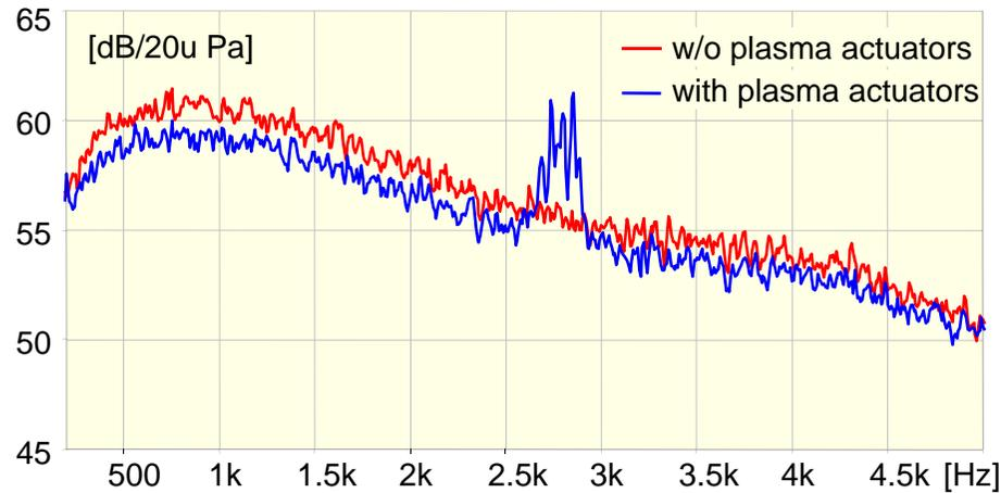
The concept is based on direct control of noise radiation by Dielectric Barrier Discharge (DBD). Vlasov–Ginevsky effect.
